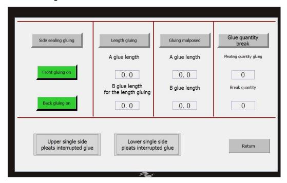
Side sealing gluing: glue the edge of the origami filter material;
