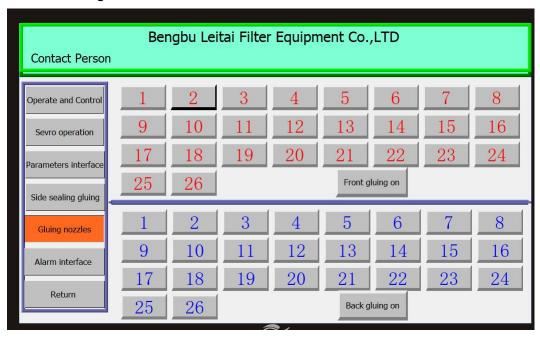
This interface is the glue head selection interface, the default is that all the glue heads are not open, only when the corresponding valve number is pressed, it means that the valve of this number is selected, when the set of valve switch is opened, the selected valve will work when the paper.
